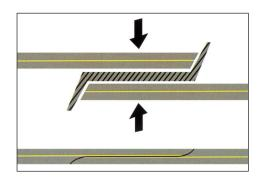
Welding by overlapping the ends of the belt. Fits all profiles in the range:
