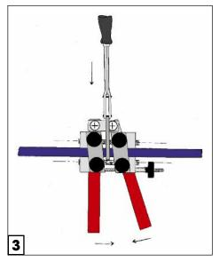
Slide the blade in between both ends of the belt and make sure that the blade bears on the whole surface to weld.
